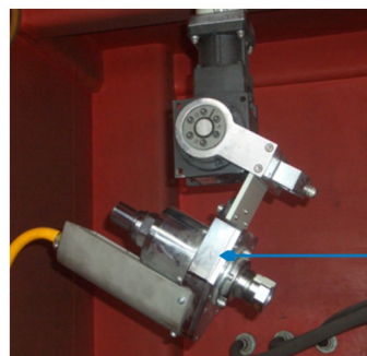
Rotary Internal Peening lance for small bores
