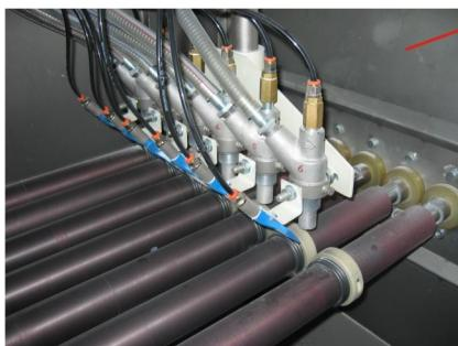
6 gun configuration for blasting 6 rollers
